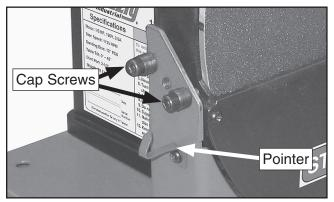
Figure 7. Location of cap screws and pointer.
